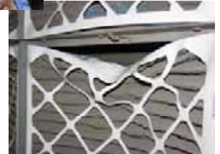
Moisture damage and microbial growth on pleated filters.
