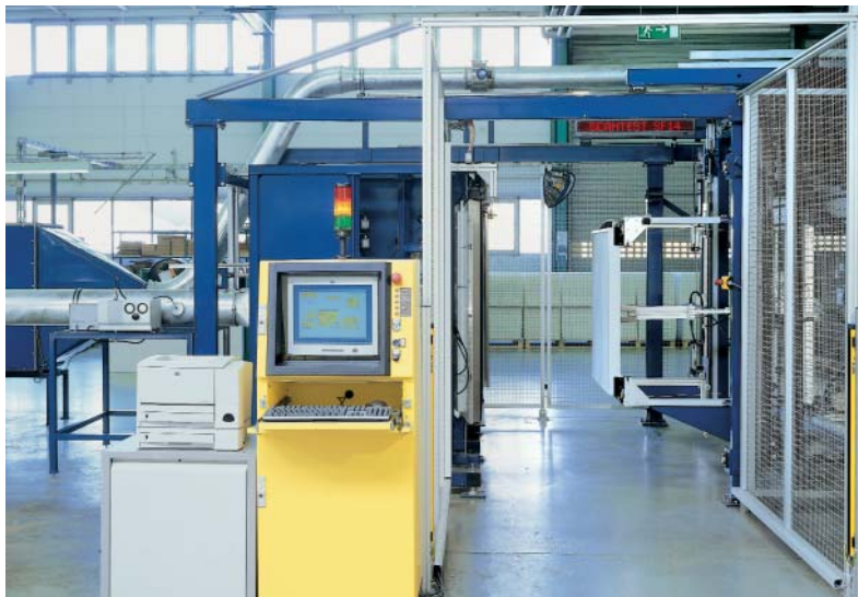
Scan test rig for individual testing of filters from Class H13
