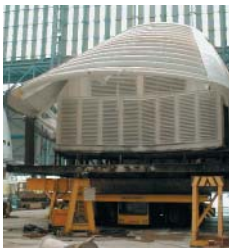
An assembled intake air filter housing, with an up-stream water separator
