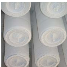
Porous ice layers on the TFP 95s at -21^{\circ}\text{C}
