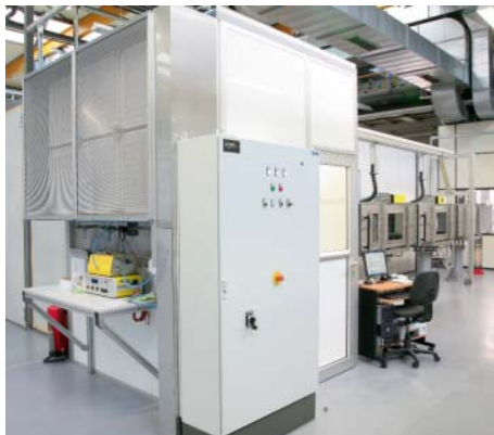
Filter test channel to EN 779 in Freudenberg's metrological laboratory
