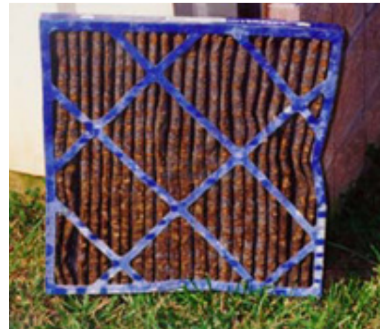
▲ Moisture damage and microbial growth on an inferior product
